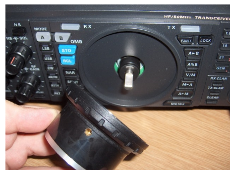
Fig 4. Remove the VFO knob to reveal the non-metal washers, two steel wavy washers and the plastic end piece on the VFO shaft...
