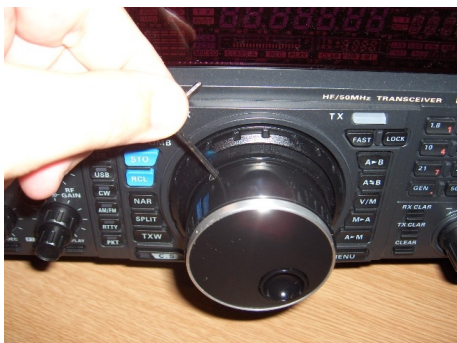
Fig 3. Insert a metric 2mm Allen key in the single hole of the VFO knob and loosen the set screw slightly – Just enough so the VFO knob can be removed...
